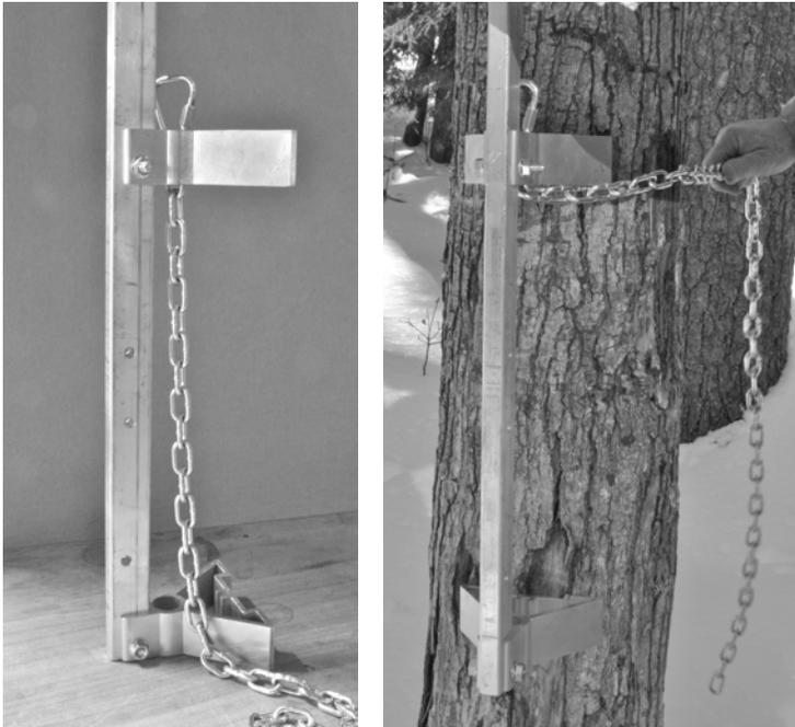
2) Wrap chain under foot and put the tightest link of chain over the bolt end, tuck excess chain down through foot. Work chain and Woodchuck down the tree if necessary to tighten against tree.
